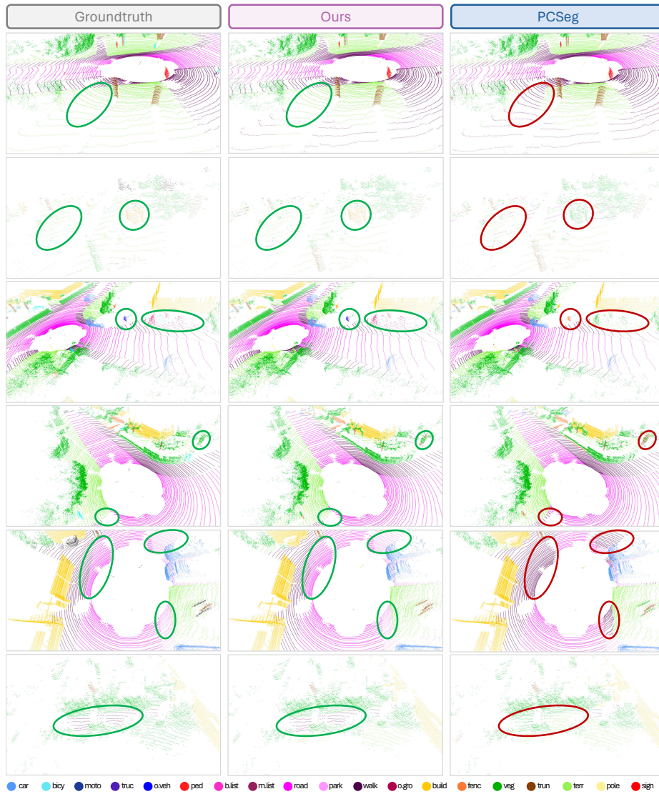
Fig. F3: Magnification of regional details: comparing with PCSeg [10] and groundtruth on SemanticKITTI [2] validation set. To highlight the differences, areas of improvement are highlighted in green, and areas of underperformance in red. Best viewed in colors.
