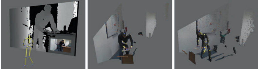
Fig. 3 (Left) The 3D skeleton obtained by Microsoft Kinect with the corresponding depth and color images. (Middle and Right) Two views of the 3D point cloud together with the obtained 3D skeleton
