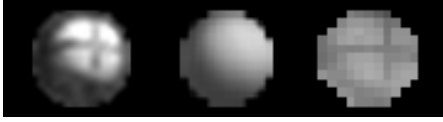
Fig. 3. The segmented image of the ball from the video (left), the average intensity of the ball region throughout the video (middle), and result of subtracting the average intensity from the original image (right)
