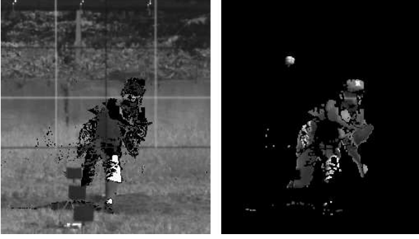
Fig. 1. The background image calculated from the video (a), and the extracted foreground (b).
